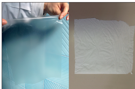
Fig. 4 Matrices made by the use of chitin nanofibrils. On the right non-woven tissue and on the left film.
