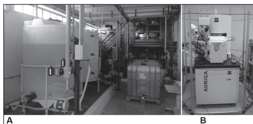
Fig. 13 New technological equipment to produce and control Chitin Nanofibrils. A: the pilot plant; B: SEM.
